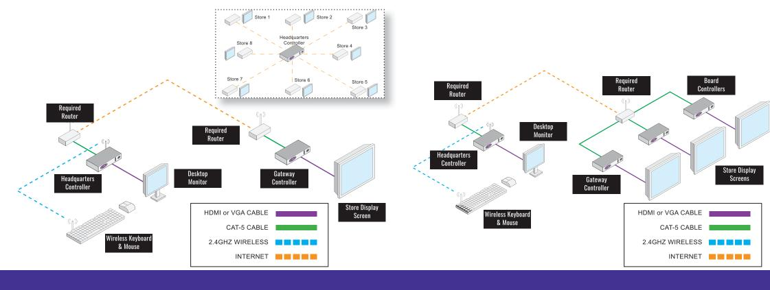
The most appropriate configuration for multiple stores, is the multi-store structure. The headquarters controller usually resides at the main office to manage slides and scheduling for all
