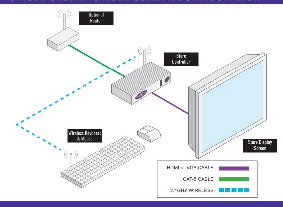
Router Switch/Hub Controllers Store Store Display HDMI or VGA CABLE CAT-5 CABLE 2.4GHZ WIRELESS
