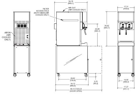
FIGURES IN BRACKETS INDICATE MILLIMETERS / DECIMAL AND FRACTIONAL DIMENSIONS EQUAL TO ( PLUS OR MINUS 1/16 INCH [1.5mm] / "WATER COOLED ONLY ).
